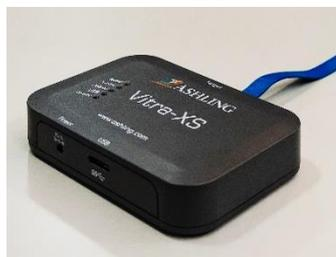
**Vitra-XS** Debug and Trace Probe: Designed for embedded developers, this probe supports multiple target architectures, including RISC-V systems with N-Trace or E-Trace, and Arm systems using CoreSight™ trace technologies (ETM, PTM, etc.). It integrates seamlessly with Ashling's recently enhanced **RiscFree™** debugger, now featuring new **Profiling, Code-coverage and Dynamic Function-flow Timeline views**.
